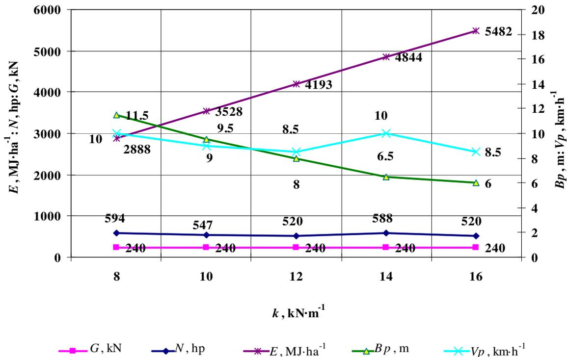
Fig. 4. Depending on the total energy costs, parameters and modes of operation of the unit on the specific resistance of the soil snarl
