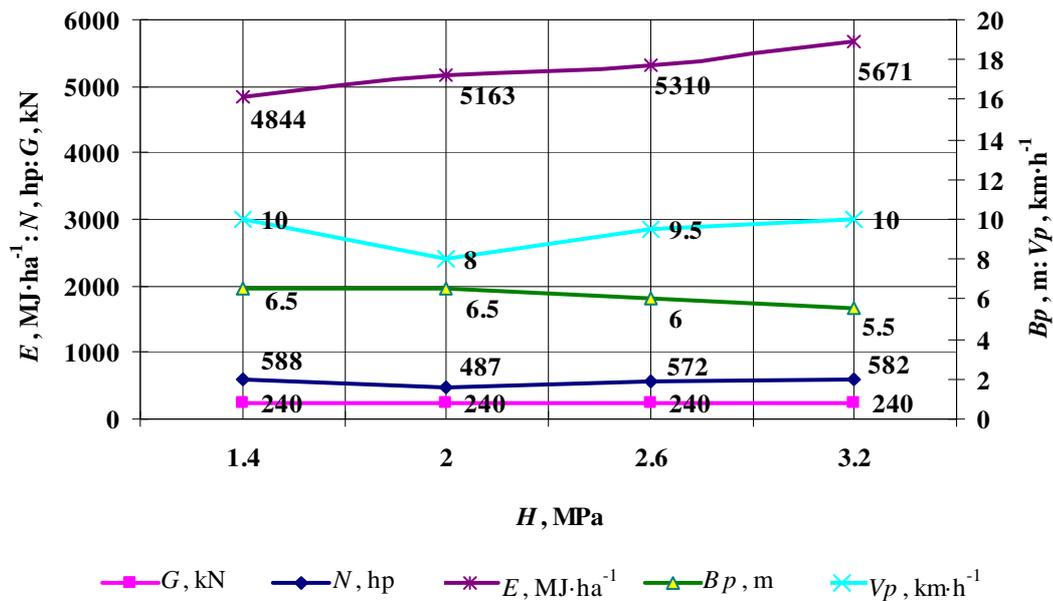
Fig. 5. Depending on the total energy costs, parameters and modes of operation of the unit on the hardness of the soil
