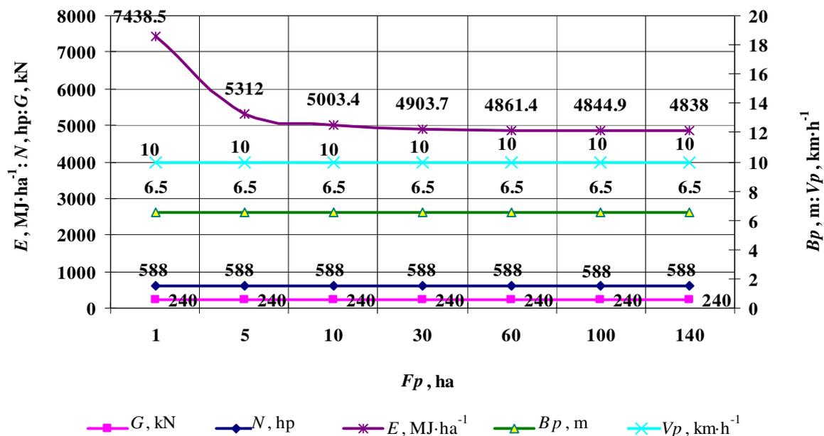
Fig. 2. Depending on the total energy costs, parameters and modes of operation of the unit from the area of the field being processed
