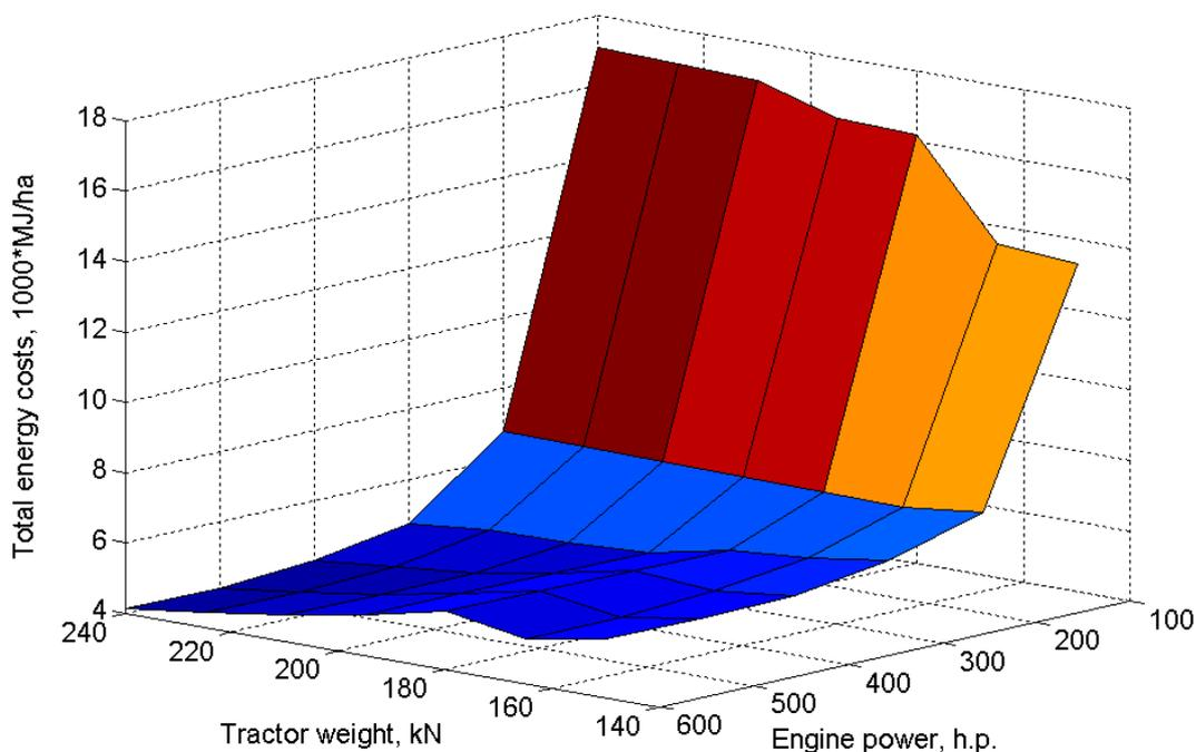
Fig. 1. Graph of the dependence of total energy costs in thousands.  $\text{MJ}\cdot\text{ha}^{-1}$  from the weight (cn) of the tractor and the power of its engine in hp
